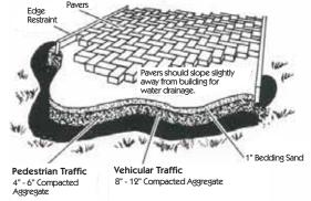
With a properly prepared sub-grade and base, a sand set installation is suitable for all types of pedestrian and vehicle traffic installations.
